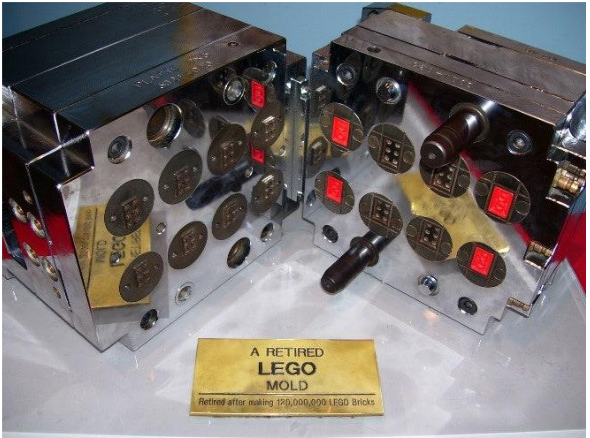
This 8 cavity mold was retired after making 120,000,000 LEGO bricks.
